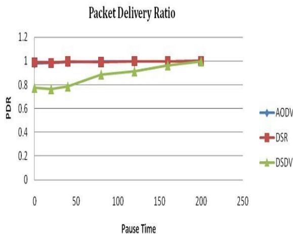
Figure 4: Impact of Pause Time on Packet Delivery Ratio for MANET Routing Protocols
